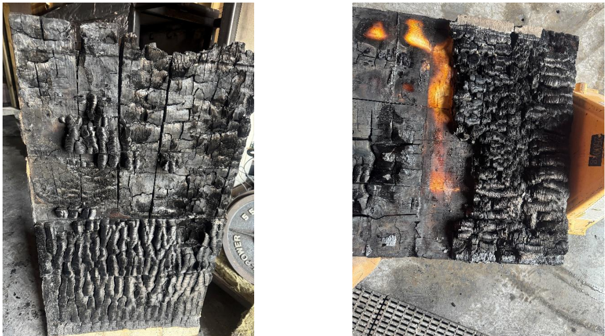
Figure 29 Wall and Ceiling samples post-test with some char cleared for measurement
