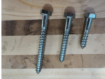
Figure 35 M12 embedment test Hex Coach Screw fixings
