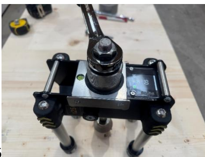
6 Figure 33 Load pull out equipment
