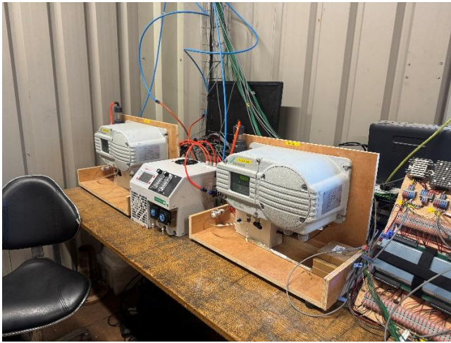
Figure 11 Gas analysis and conditioning system
