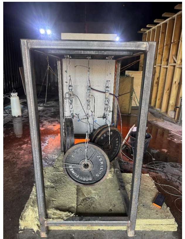
Figure 18 Loading end of rig with static weights
