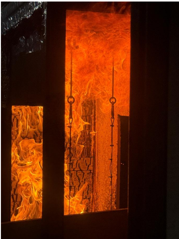
Figure 20 Loaded fixings under fire
