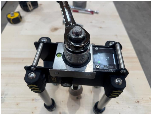
Figure 24 Load pull out equipment
